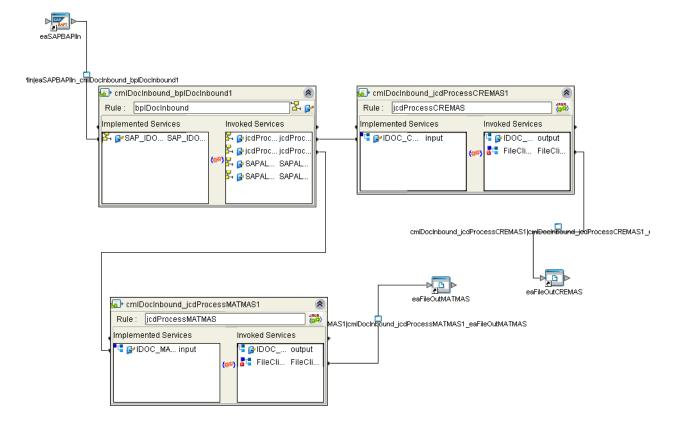
Figure 84 Connectivity Map - Binding the JCD Components
